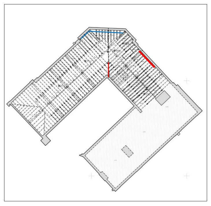
Figure 41. Showing the roof plan. Areas marked in red show where we exposed the decayed wallplate at the underside and decayed valley rafter. The area marked in blue shows the previously repaired wallplate.
