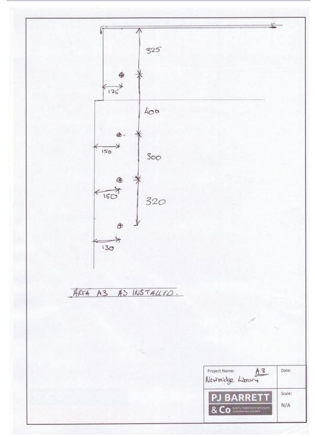
Figure 22. Showing a site sketch of the stitching works Detail A3 looking West.
