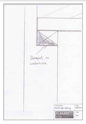
Figure 10. Site sketch showing the decay at the wallplate where it was opened up.
