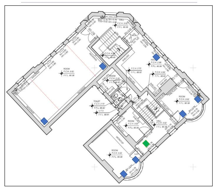
Figure 40. Showing the first-floor plan. We have marked up the areas opened up by PJ Barrett in Blue and in green, where we opened up a new hatch to access the attic. The Red dashed line represents the approximate location of the steel UB sections supporting the floor joists.
